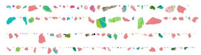
Figure 2. False-colour particle map from a sample from the Bushveld Complex UG2 Reef.
