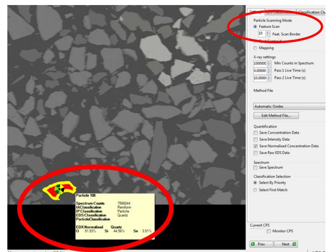
Figure 7: Screenshot of "Feature Scan" functionality within a Mineralogic® system.
