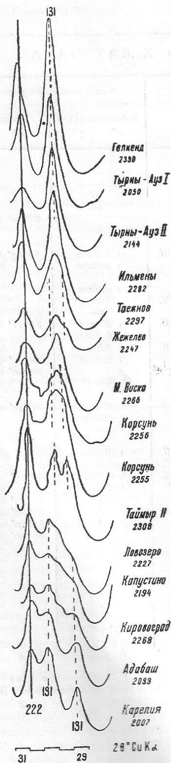
Fig. 1.—Diffractometer records in the region of the 131-131 reflections, to show triclinicity of the investigated specimens.
